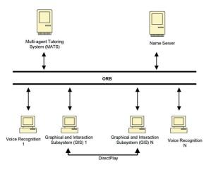
Figure 4 MAEVIF's System Architecture.
